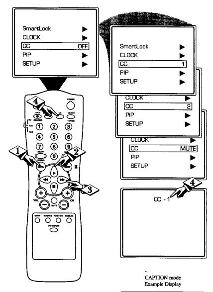
NOTE: The CC-MUTE option can be used to set the TV to turn the Closed Caption mode "ON" whenever the MUTE button on the remote is pressed. This activates the CC-1 option. MUTE will appear smaller in the upper center of the screen.
